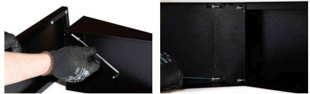
Fix the lateral supports to the front using the screws supplied
